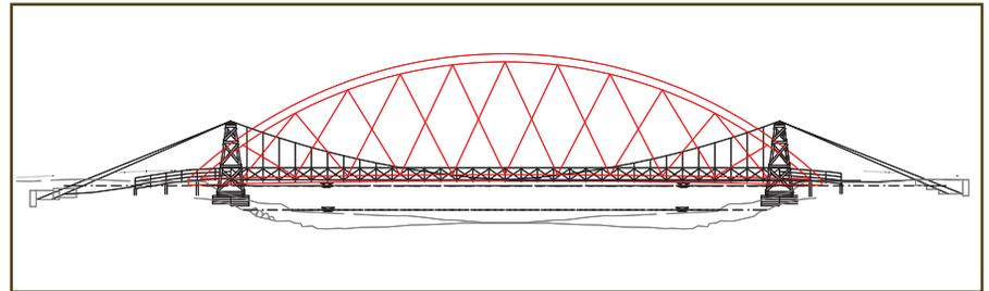
**Note: Existing bridge shown in the background is for comparison to height of the proposed bridge.**
